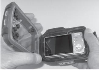
Step 4: Close housing and push down on latch as shown to firmly seat latch into housing.
