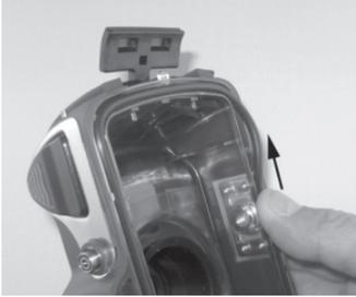
Step 2: Gently lift and remove O-ring from its groove.
